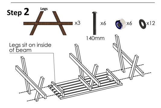
Tighten nuts and bolts with spanner and allen key.
